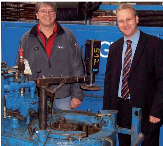
Udo Boerrigter, the general manager of GTS, and Leine & Linde sales engineer Andreas Frochte, behind the 7 5/8" hydraulic tongs with a revolution counter. It is centred around an ATEX 632 encoder.
